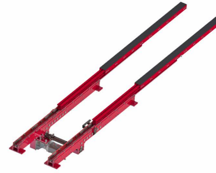
单电机单伸位窄叉 (HFTB100x125-H-SM-2Z) Single motor single extension narrow fork(HFTB100x125-H-SM-2Z)
